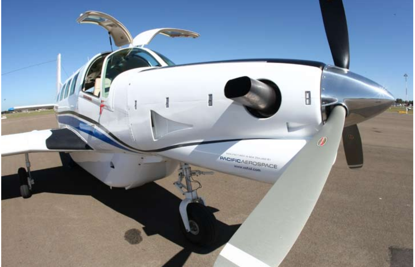
SON OF CRESCO Little of the Cresco's design survives in the P-750, with the wings, ailerons, flaps, and fuel system all replaced or modified.
