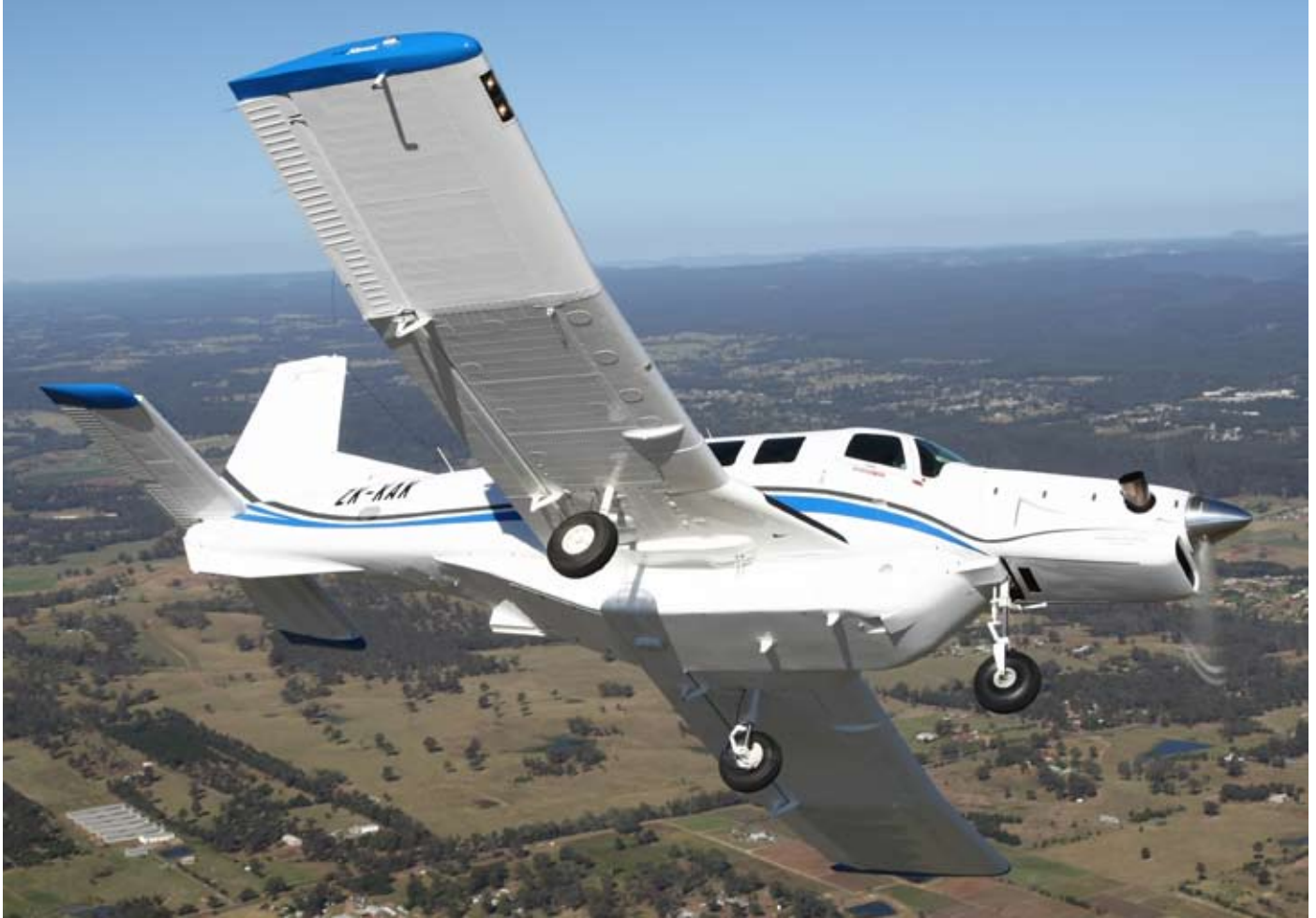
SKYDIVING ORIGINS The P-750 was first conceived in 1999 when US skydiving companies approached Pacific Aerospace seeking an enlarged version of the Cresco that could carry up to 17 skydivers to altitude and return to the point of departure in approximately 15 to 16 minutes. US FAA certification was awarded in 2004.
